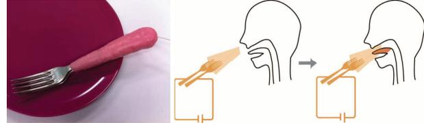
**Figure 3. Polar opposite circuit to add electric taste to food**
