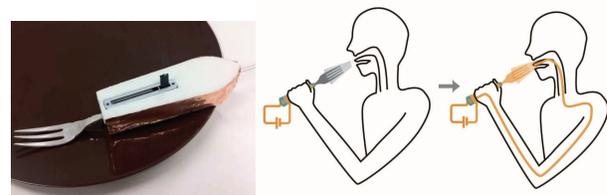
**Figure 4. Single-pole circuit to add electric taste to food**
