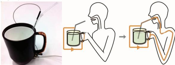
**Figure 2. Single-pole circuit to add electric taste to drink**
